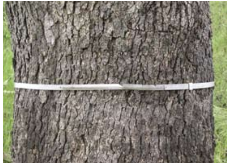
Figure 7. Dendrometers, such as this one on a blue oak, facilitate precise measurement of a tree's radial growth. A stainless steel band held together by a spring expands along with the tree. The expansion is measured using notches on the band.
